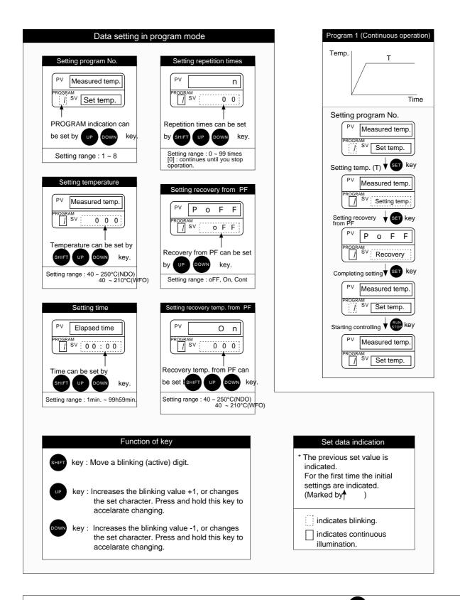
Press key to check the set value or the measured value while controlling. And then if you press operative, temperature, time, repetition time, recovery from power failure or recoverying temperature from power failure can be checked by every pressing operative, key. When the unit is left for more than a minute without any key operation, the indication returns to the previous setting automatically.
