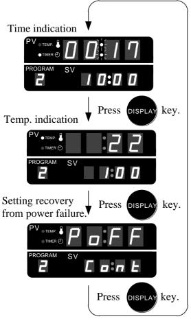
Displays after count up of time is changed as follows. If the unit is left for a minute without any key operation, the display changes to the previous indications automatically.
